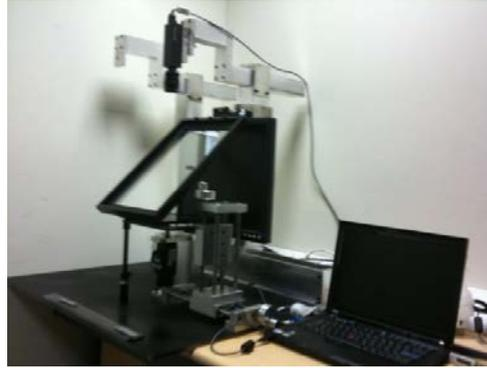
Figure 4 (a) Schematic of Phase Shift Reflectometry
